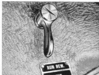
This switch cannot be moved from "run" to "rewind" or vice versa while the current supply switch is on. This interlocking assures correct operation
