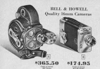
A Bell & Howell "70-DL" Roll-load 16mm Turret Camera. Top quality 3-lens turret camera for the serious amateur or professional. Uses economical double or single perforated roll film. Critical through-thelens focusing. Viewfinder adjusts for parallax. holds accessory objectives to match accessory lens fields. Extra-long 22-ft. film run. Hand crank for extended run, backing up film, lap dissolves, etc.
