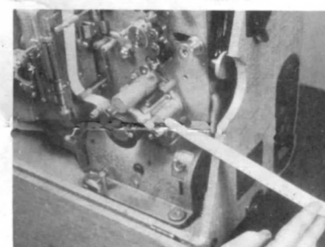
10. . . . move film horizontally to bottom of sprocket, threading between trip levers and under sprocket.
