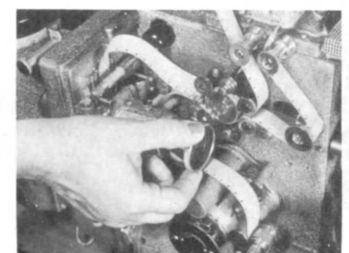
21. To focus image on screen turn lens until sharp; then tighten lens lock screw.
