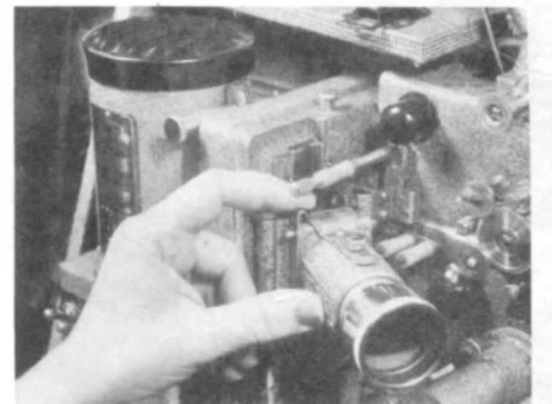
2. Open swing-out lens by pulling on release latch shown at index finger.
